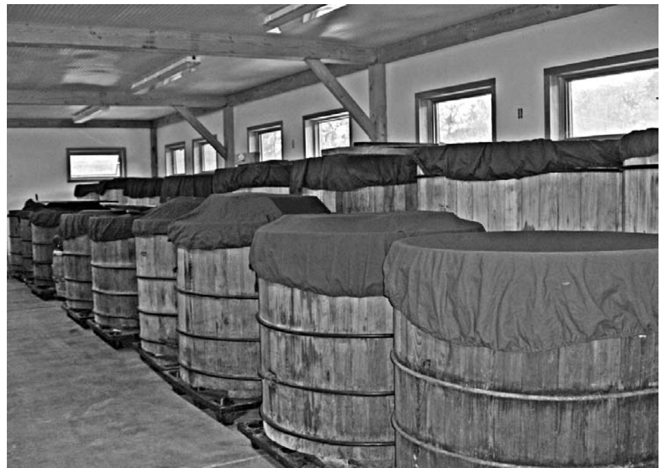
Miso vats lined up in our new timber framed storage building. The fermentation vats are made of American Cypress. Ten smaller vats, built in 1979, each hold about 2400 pounds of miso. Seventeen larger vats, built over the past two decades, each hold about 7600 pounds of miso. The miso ages in these vats from three months to three years depending on the variety. Radiant floor heat supplied by a wood burning furnace keeps the miso warm during the winter months.
